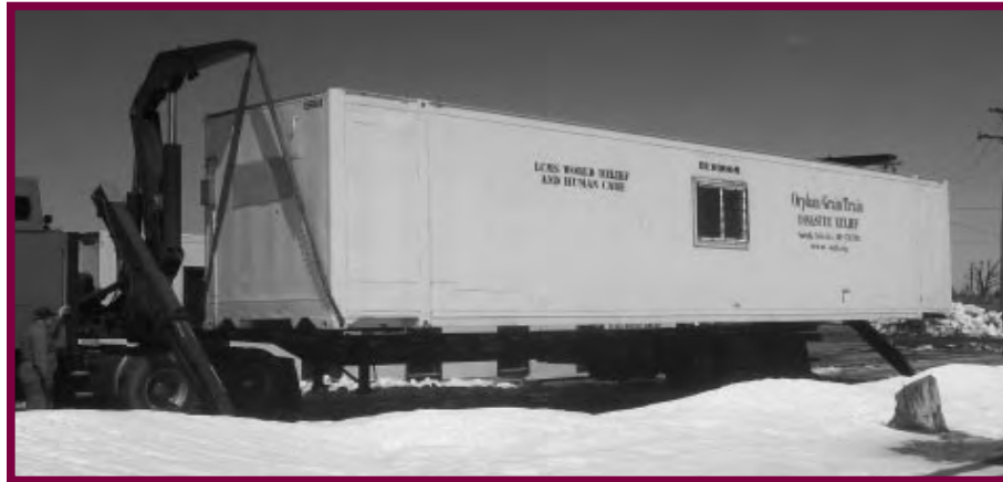
The Orphan Grain Train has become proficient at converting shipping containers into bedroom, shower and storage facilities. Here, Orphan Grain Train's Hammar trailer lifts a volunteer village bedroom unit at Greensburg, Kansas.
